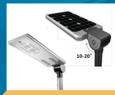
The system is provided with battery storage backup sufficient to operate the light for 12-14 hours per night. The system is provided with automatic ON/OFF time switch for dusk to dawn operation and overcharge / deep discharge prevention cut-off with LED indicators. The systems electronics provide for over-charge and over-discharge cut-off, essential for preventing battery and luminaries damages.
